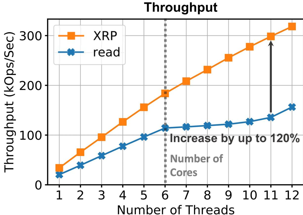
XRP can scale well even if the number of threads exceeds the number of cores
