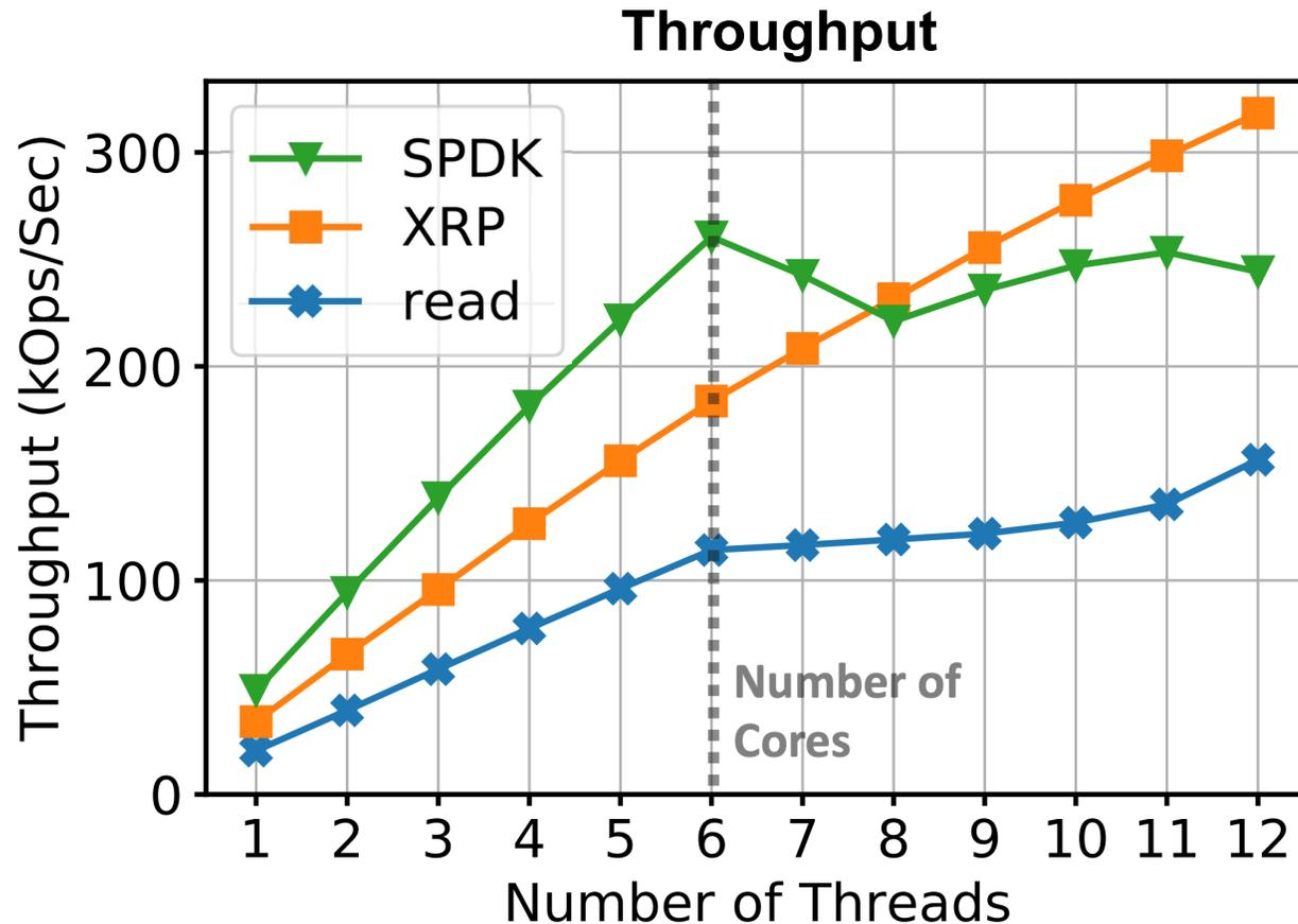
SPDK fails to scale beyond 6 threads because SPDK threads cannot yield CPU when waiting for I/O to complete
